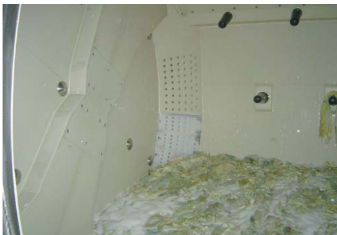
The extremely smooth drum interior due to polypropylene construction.
